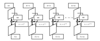
Figure 1 Fundamental procedure of Greyworld-based white balance for video capture
