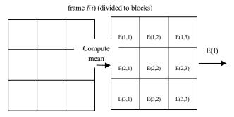
Figure 2 Illustration of block-based computation of means
